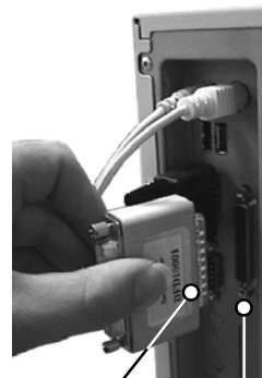
25 pin D male connector on security key (dongle). 25 pin D female connector fitted to computer (back) panel.
